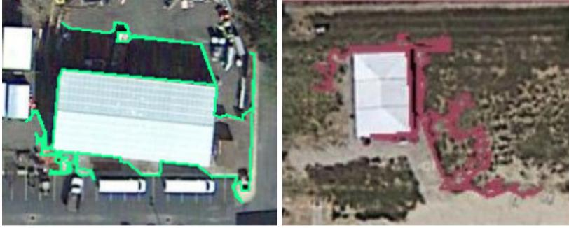
Fig. 6: Example of contours that overdetected a candidate. The green and red lines are the contour lines. The bounding boxes can be repositioned to detect these buildings.
